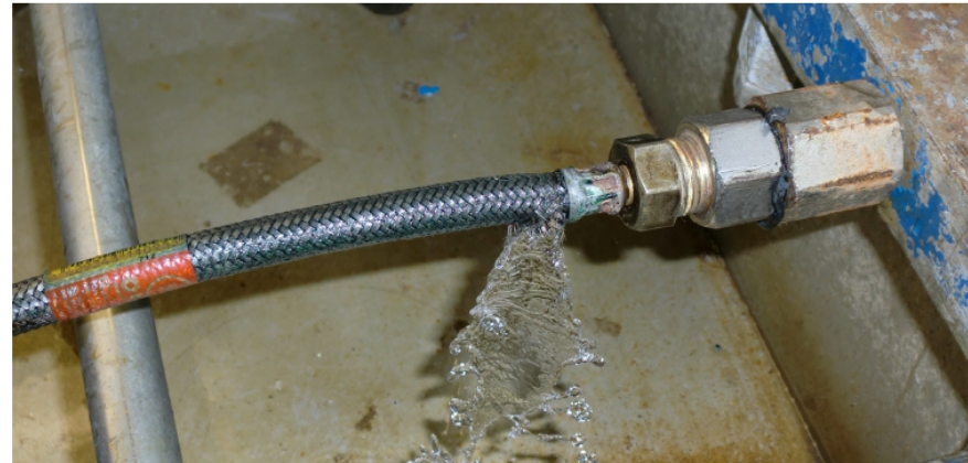
STAINLESS STEEL BRAIDED HOSE BURST PICTURE RESULT: 20 BAR (TEST FAILS)
