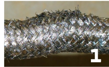
Magnified detail of the deteriorated braid before pressure test is run.
