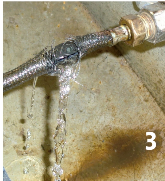
Magnified detail of the deteriorated braid before pressure test is run.
